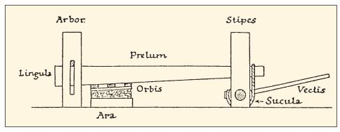
Fig. 9. Cato's lever-and-drum press (Frankel 1999: fig. 8)
