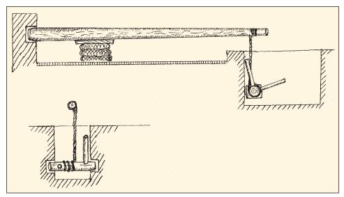
Fig. 5. Reconstruction of lever-and-drum presses from Moshav Habonim
